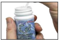
Press (READ) to initiate a 20 second countdown and simultaneously **DIP** the test strip by submerging all pads in the sample then use a gentle constant back and forth motion (2 strokes per second) until the timer displays "1". Remove and discard the strip.
