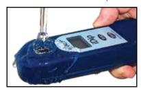
Press READ to initiate a 20 second countdown and simultaneously **DIP** the test strip by submerging all pads in the sample then use a gentle constant back and forth motion (2 strokes per second) until the timer displays "1". Remove and discard the strip
