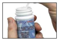
Rinse the cell 3 times with the water sample to be tested and **FILL** to the top to begin test.
